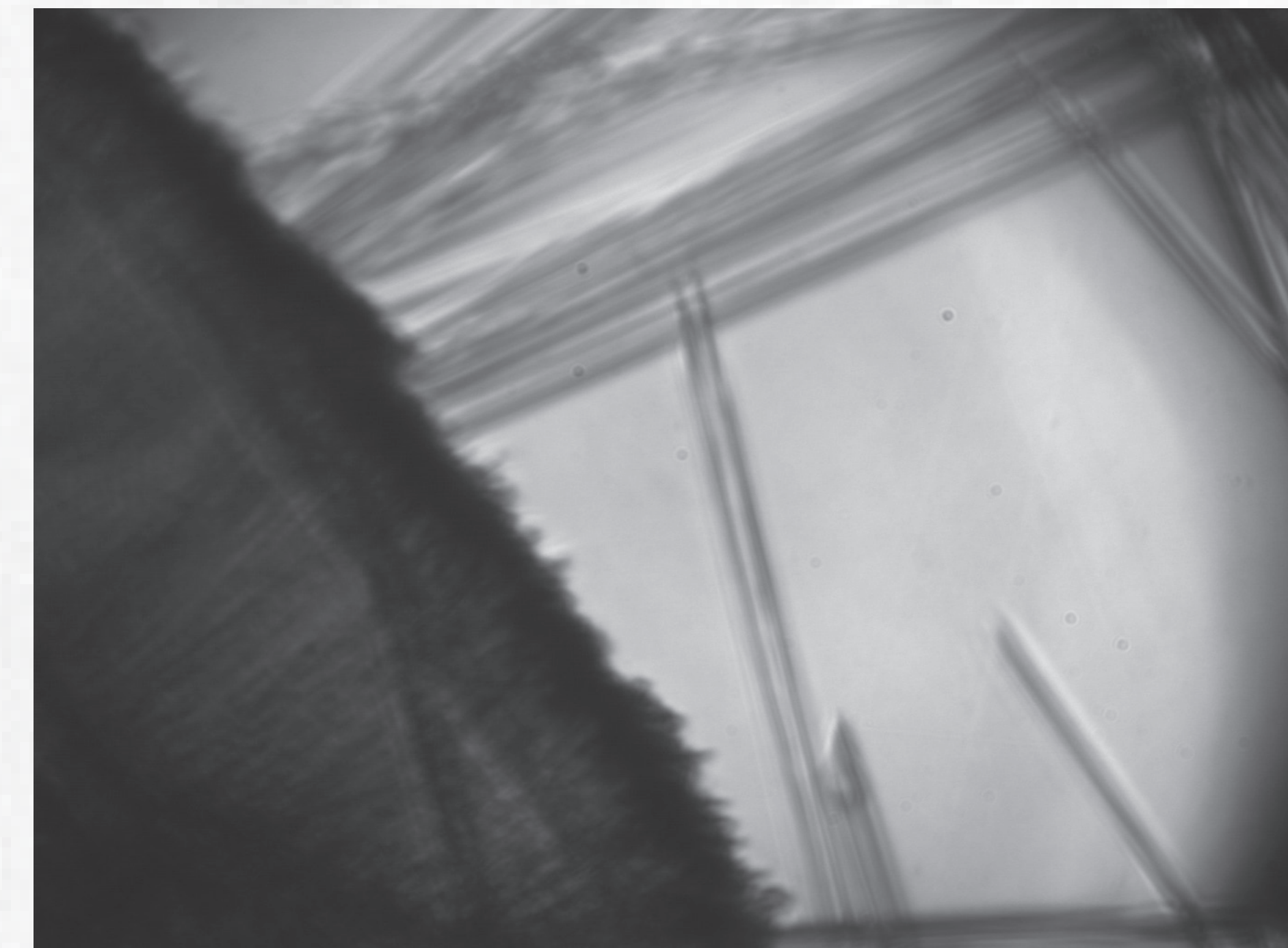
Figure 6: Image taken during the solidification of a methanol-water solution at T = 201 K and p = 314 MPa. The original thin Ice-II crystals are visible against a clear liquid background, with a solidification front approaching from the lower left-hand side of the image. The image is approximately 1 mm across.
