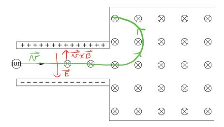
a. (10 pts.) What is the speed of an ion which passes through the velocity selector undeflected?
