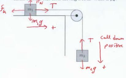
To solve with  $2\vec{F} = m\vec{a}$ 1st find  $a_1$   $N_{1p}^2 = N_{1s}^2 + 2a_1\Delta N$   $A_1 = \frac{N_{1p}^2 - N_{1s}^2}{2\Delta N}$   $A_1 = \frac{0 - (0.960 \text{ m/s})^2}{2(2.00 \text{ m})}$   $A_1 = \frac{0 - (0.960 \text{ m/s})^2}{2(2.00 \text{ m})}$
