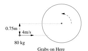
4. (30 pts.) A merry-go-round (a disk of radius 1.8 m and moment of inertia  $300 \text{ kgm}^2$ ) is rotating freely at an angular velocity of 0.75 rad/s in the direction shown in the diagram. Daredevil Dave (whose mass is 80 kg) runs along the path shown in the figure with an initial speed of 4 m/s and jumps onto the **edge** of the merry-go-round as shown. Your ultimate goal will be to find the final angular velocity of Dave and the merry-go-round together.
