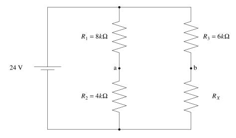
a. (15 pts.) If the voltage difference  $V_{ab}$  is measured to be 0 V, what is the unknown resistance  $R_X$ ?
