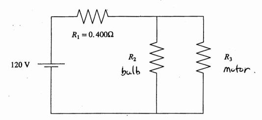
a. (15 pts.) When the motor is off (or disconnected), a total current of 0.626 A passes through  $R_1$ . What is the power dissipated by the light bulb?
