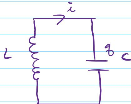
$$\begin{aligned} L &= 85.0 \text{ mH} \\ C &= 3.20 \mu\text{F} \\ i_{\max} &= 0.850 \text{ mA} \end{aligned}$$
