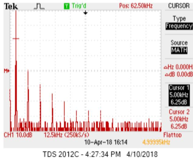
Figure 1: Oscilloscope display for FFT of an input 5000 Hz triangle wave on the TDS2012C oscilloscope. (See Fig. 2 for a similar image for the TBS-1000C oscilloscope.) Both cursor 1 and cursor 2 are set on the fundamental, which has a frequency of 5.0 kHz and an amplitude of 6.25 dB. Note the successive peaks at 15.0 kHz, 25.0 kHz, *etc.* These amplitude measurements were made with the **Flattop** window.
