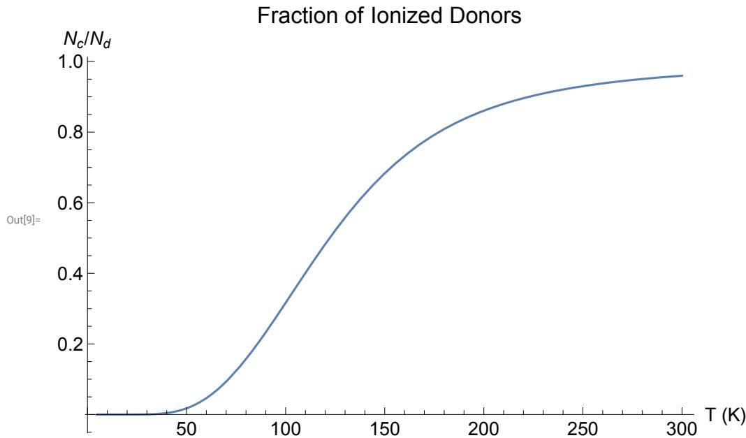
At room temperature, nearly all of the donors will be ionized. The temperature at which half of them will be ionized is about 122 K:
