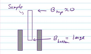
If X = positive (paro magnetic) the matrial is attracted into the region of strong field Equivalently, the magnets are pulled up.
