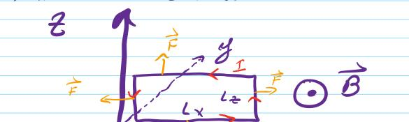
Net F = 0 in a uniform B. (Torque is not zero -> current loop tendo to align with B.)
