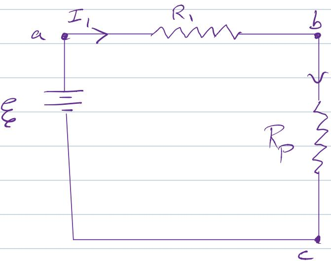
$$\frac{1}{R_P} = \frac{1}{R_2} + \frac{1}{R_3} = \frac{1}{2k\Omega} + \frac{1}{3k\Omega} = \frac{5}{6k\Omega}$$
