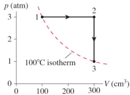
102. || A monatomic gas follows the process  $1 \rightarrow 2 \rightarrow 3$  shown in Figure P12.102. How much heat is needed for (a) process  $1 \rightarrow 2$  and (b) process  $2 \rightarrow 3$ ?
