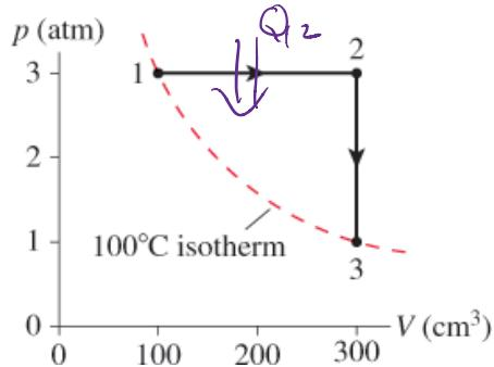
$$\begin{aligned}P_2 &= 304,000 \text{ Pa} \\V_2 &= 3V_1 = 3.0 \times 10^{-4} \text{ m}^3 \\T_3 &= 3T_1 = 1119 \text{ K}\end{aligned}$$
