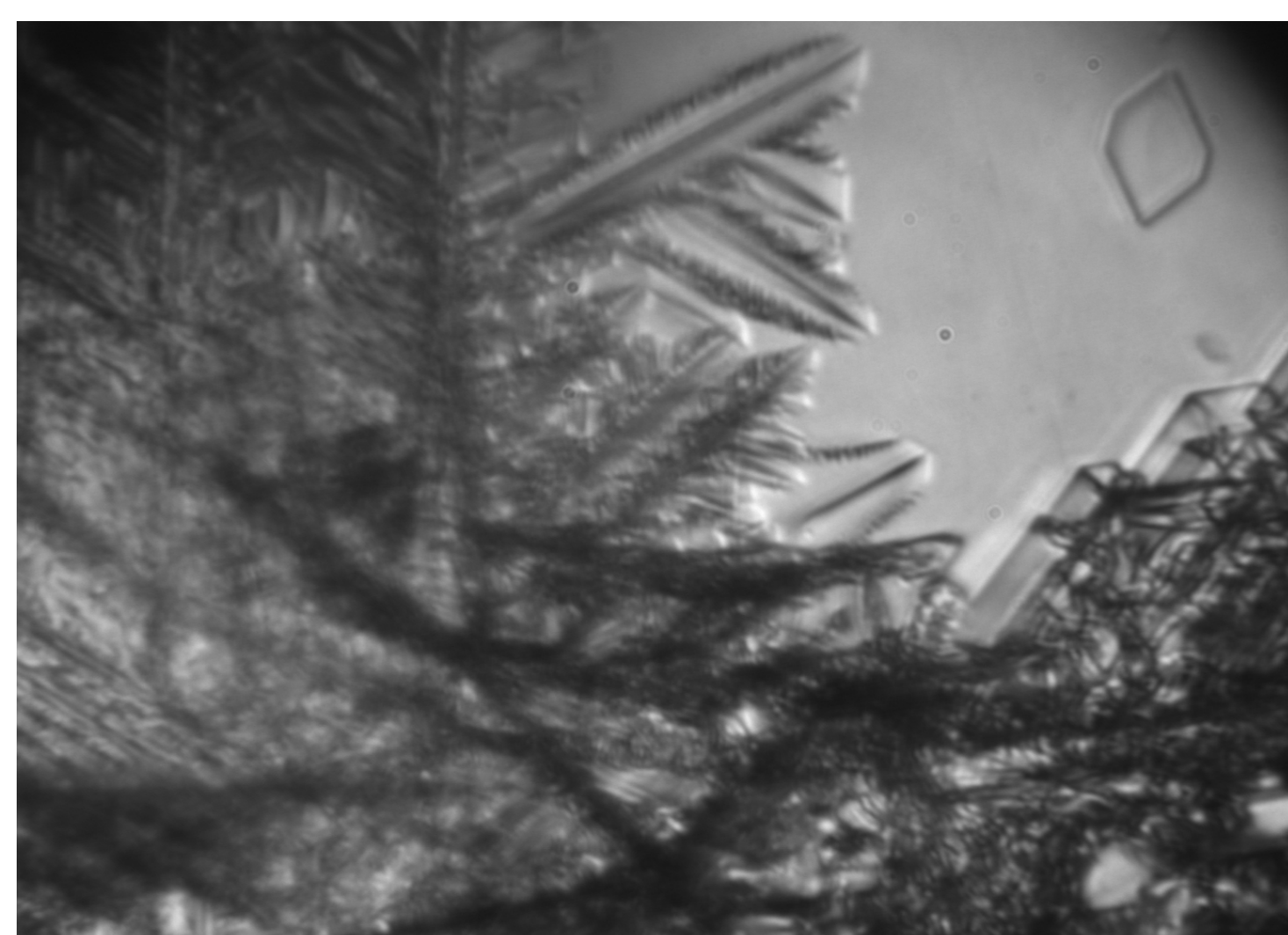
Figure 4: Ice-Ih crystals growing during the freezing of a methanol-water solution at a temperature of 254 K and pressure of 50 MPa. The image is approximately 1 mm across.
