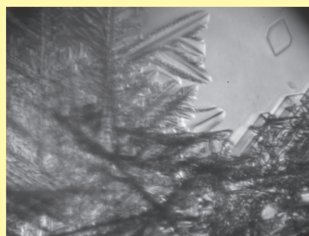
Figure 6: Ice dendrites growing at T = 225.77 , p = 49 \text{ MPa} , in a methanol-water solution.
