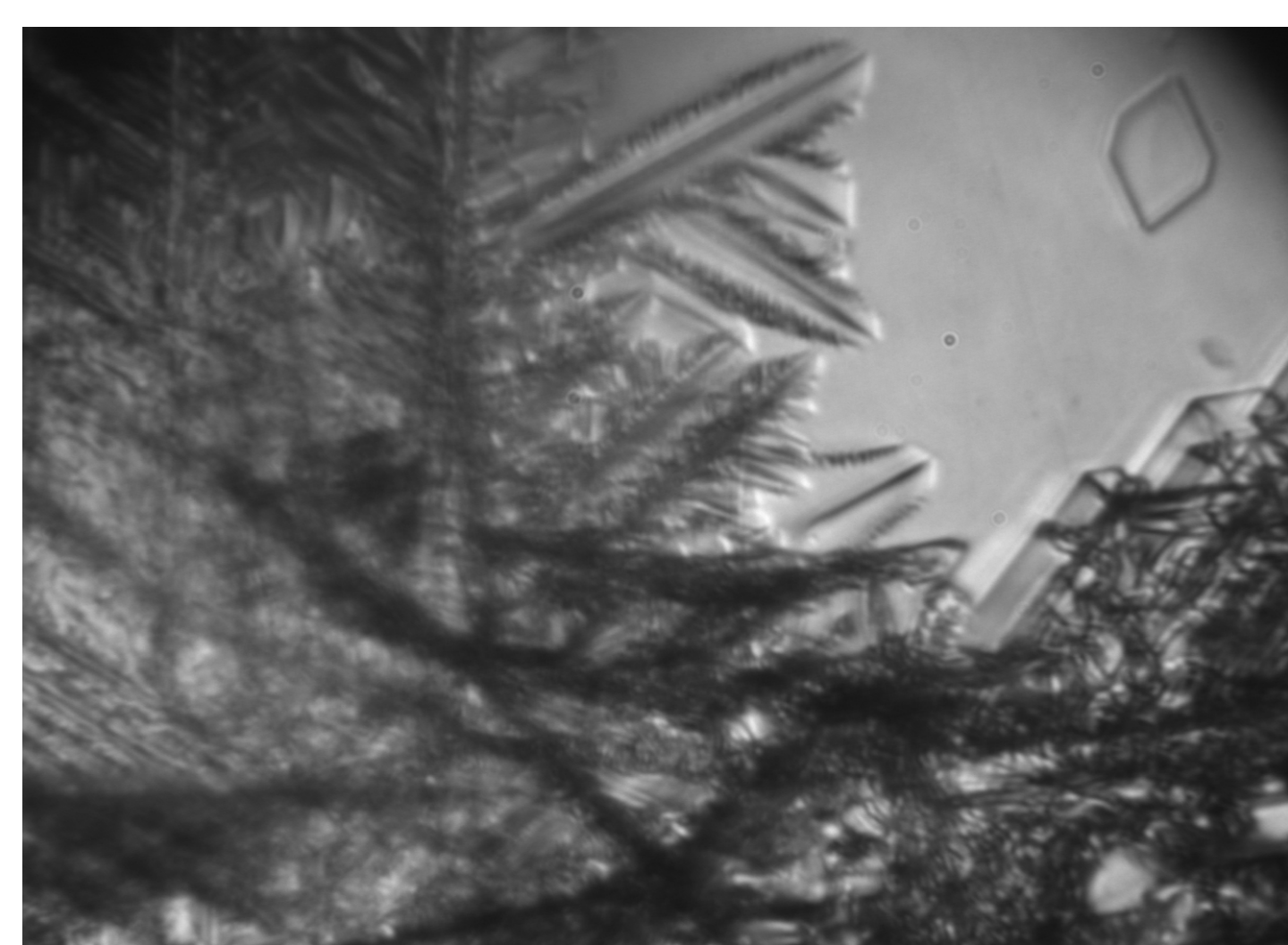
Fig. 5: Ice-Ih crystals growing during the freezing of a methanol-water solution at a temperature of 254 K and pressure of 50 MPa.
